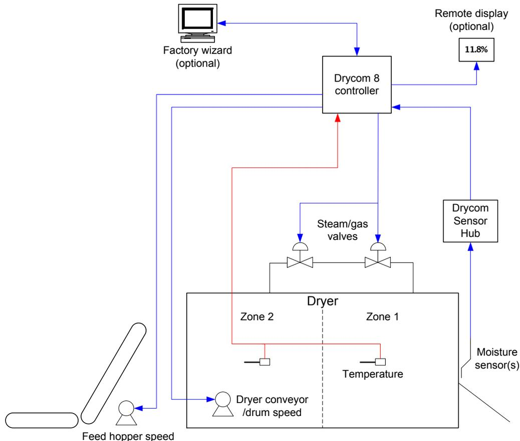
DRYCOM Moisture Control systems are precision instruments that use a unique adaptation of the conductivity principle. They are designed to operate in hostile industrial environments and provide our customers with:
